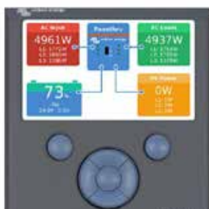
Color Control GX, showing a PV application
